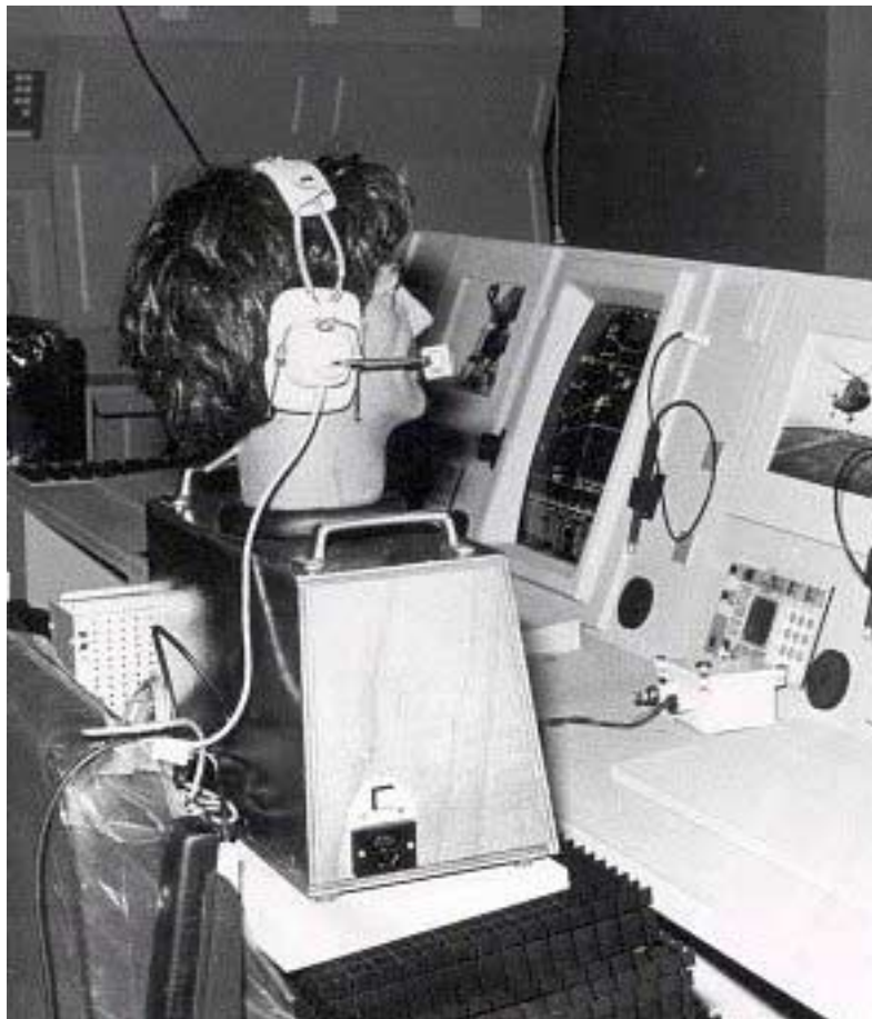
Fig. 8.3 Artificial mouth used for the assessment of microphones.
